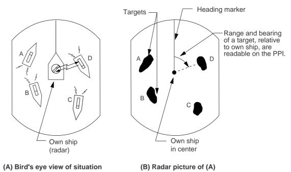
Figure 1-1 How radar works
